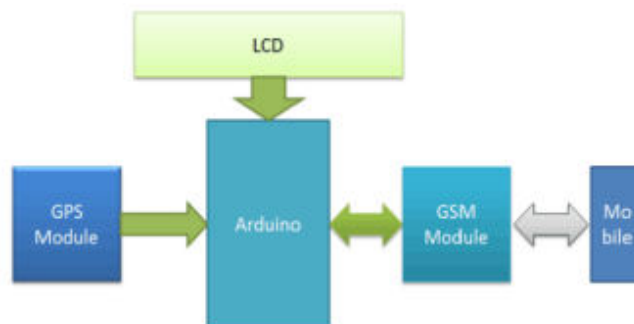
Figure.3 Block Diagram of Arduino based vehicle tracking system.
